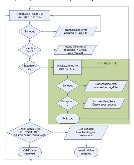
A simple example for reading out a pressure value.
