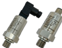
EDN.321 0.5% -1...0 & 0...0.6 to 0...1000 bar, Output signal: 0.5...4.5 / 5V ratio-metric
