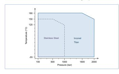
KELLER 7LHP series high pressure transducers are available with various material options. Stainless steel, Inconel 718 or titanium can be selected (see "Mechanical data") in line with requirements.
