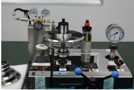
Europascal Pneumatic DWT-BA2-70 Max. 70bar
